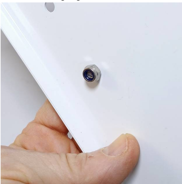
Close the holes with M5x6 Torx bolt and M5 lock nuts. If the moto seat is going to be installed, use these 4 bolts to secure the moto seat from below.
