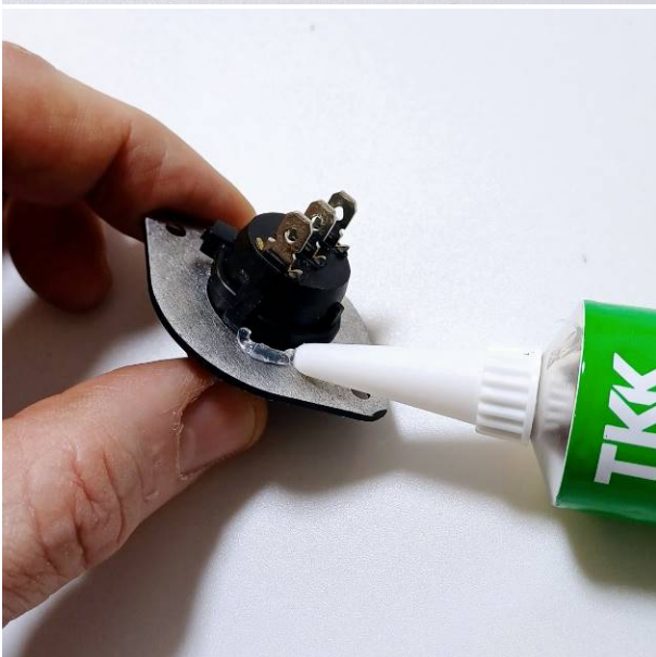
Add silicone to achieve a watertight fit.
